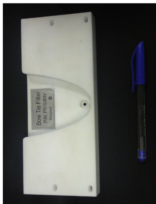
Figure 1 Photograph of typical Teflon made bowtie filter which is narrow at center and thick at the edges.
