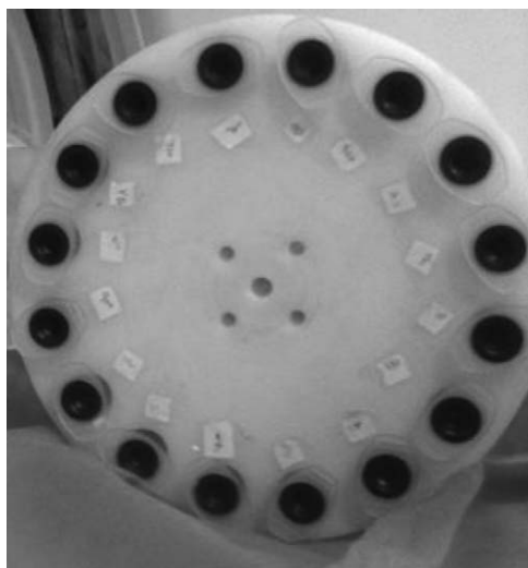
Photograph of the cylindrical polyethylene phantom consisting of 16 syringes filled with different concentrations of K_2HPO_4 solution simulating different biological tissues.
